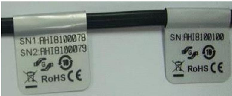
The serial number for each sensor or actuator appears listed in the web interface after each sensor or actuator is detected by the PRO3X. Match the serial number from the tag to those listed in the sensor table.
