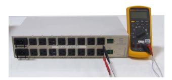
Figure 2. Measuring Branch A and B, Line 2
