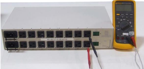
Figure 1. Measuring Branch A and B, Line 1
