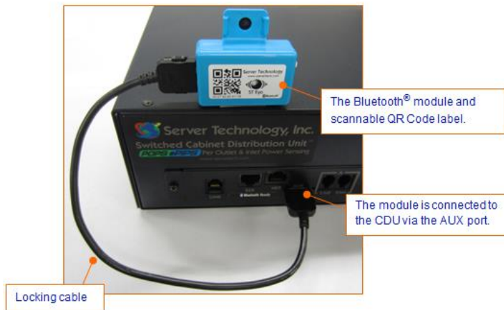
Figure 2. Bluetooth Module (showing connection to the CDU)
