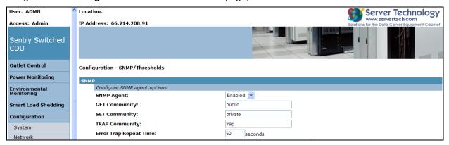
**3.** From the SNMP Agent drop-down list, select the Enabled option (shown above) and click **Apply**. The message "Value changed – restart required" displays:
