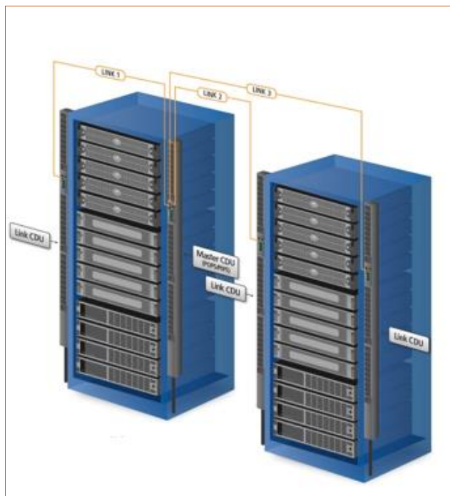
Multi-Linking View in the Equipment Cabinet
