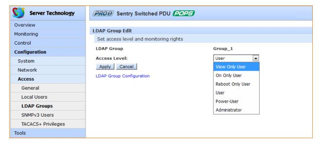
From the Access Level drop-down menu, select the desired user access level as the above screen sample shows (View Only User, On Only User, Reboot Only User, User, Power-User, or Administrator) to assign to the LDAP group.
