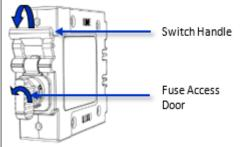
To service the fuse or turn OFF the branch, rotate the Switch Handle toward the Fuse Access Door.
