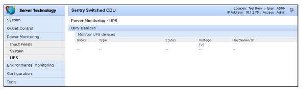
The UPS page displays all available UPS devices associated with the CDU, showing index, type, utility power state (status), nominal voltage, and hostname/IP address.
