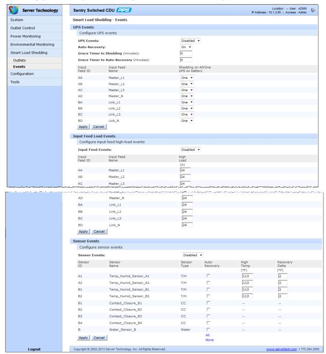
Example of Load Shedding feature for a PIPS-enabled CDU
