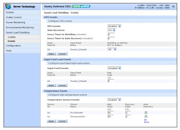
Example of Load Shedding feature for a POPS-PIPS-enabled CDU
