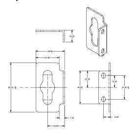
Mounting bracket assembly for one PDU
