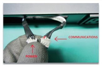
2) Slide the assembly out of the enclosure and disconnect the cables from the "old" NIC. The communications cable (J1) has three white wires and one red wire; the power cable (J8) has two black wires and two white wires (as shown above).
