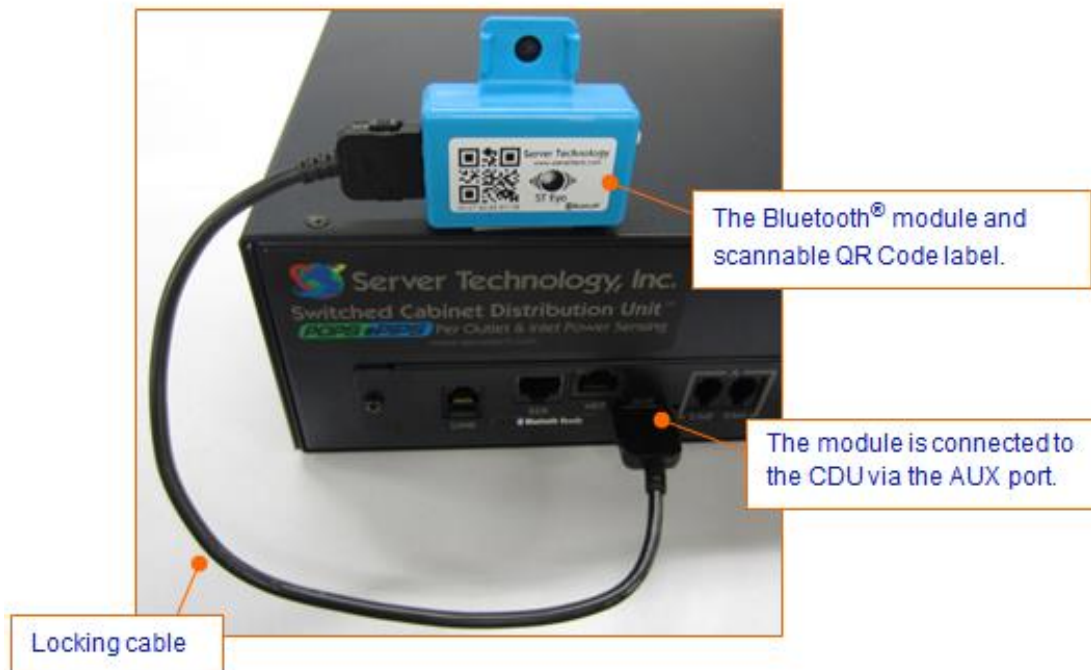
Bluetooth Module (showing connection to the PDU)
