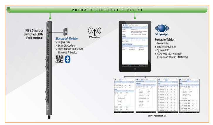
Figure 1. System Overview of Mobile Monitoring Using Bluetooth<sup>®</sup> Wireless Technology
