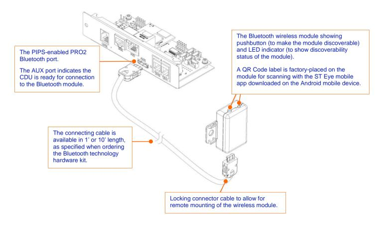
Figure 3. Hardware Connection Using Bluetooth Wireless Technology
