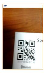
When a valid QR Code label is located, ST Eye connects to the Bluetooth modules, displays PRO2 information in the default System tab, and refreshes displayed data every 10-seconds.
