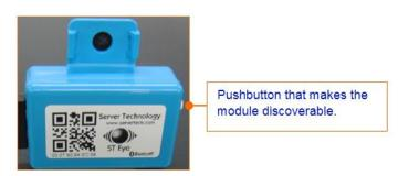
Figure 4. Close-up of the Bluetooth Module (showing QR code label and pushbutton)
