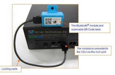
Figure 2. Bluetooth Module (showing connection to the PRO2)
