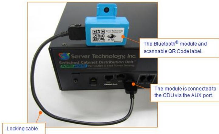
Figure 2. Bluetooth Module (showing connection to the PRO2)
