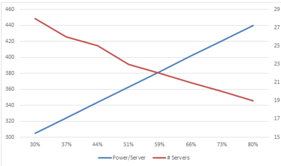
Figure 4: Power per server and Servers per rack vs. CPU usage – 30A 3-phase 208V circuit from Managing Variable Data Center Rack Densities , a white paper by Server Technology.
