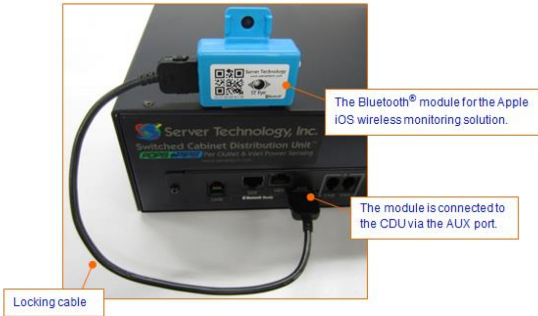
Bluetooth Module and Connection to the PRO2
