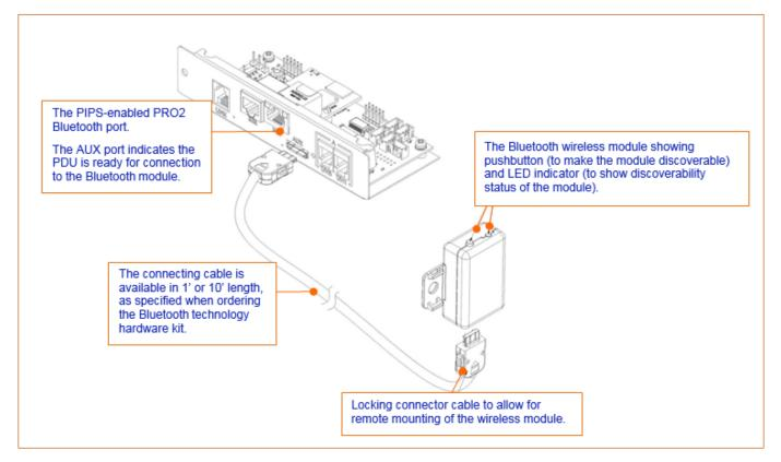
Hardware Connection Using Bluetooth Wireless Technology
