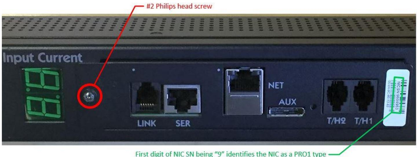
2. Slide the PROx Edge-Mount NIC directly out of the enclosure until it is just clear of the face of the PRO1/PRO2 intelligent PDU. See photo, next page.
