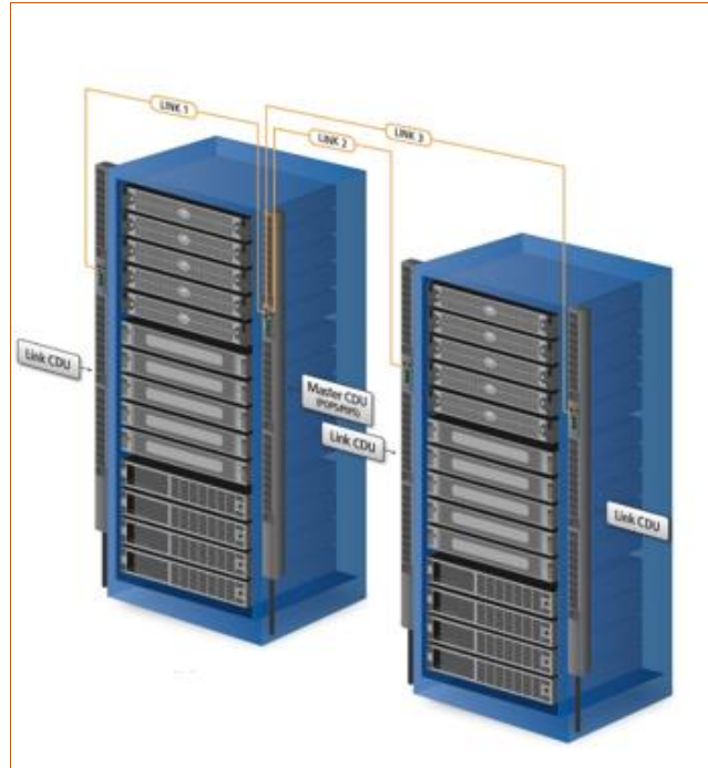
Multi-Linking View in the Equipment Cabinet
