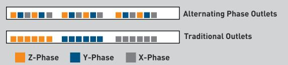
Power wiring becomes much more simplified with this type of PDU since power cords do not need to be stretched across the length of the vertical PDU to reach separate branches. Plugging into a different phase only means moving the cord several inches to the next available receptacle. Shorter power cords from the server to the PDU can now be used thus cleaning up the back of the rack cabling.
