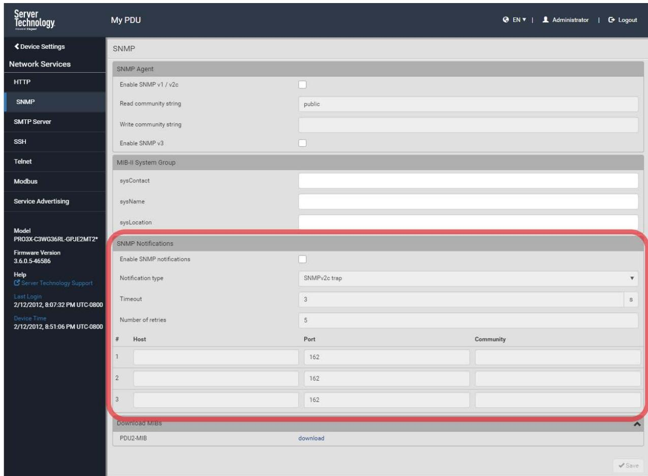
Figure 2: SNMP notification settings dialog of the web user interface
