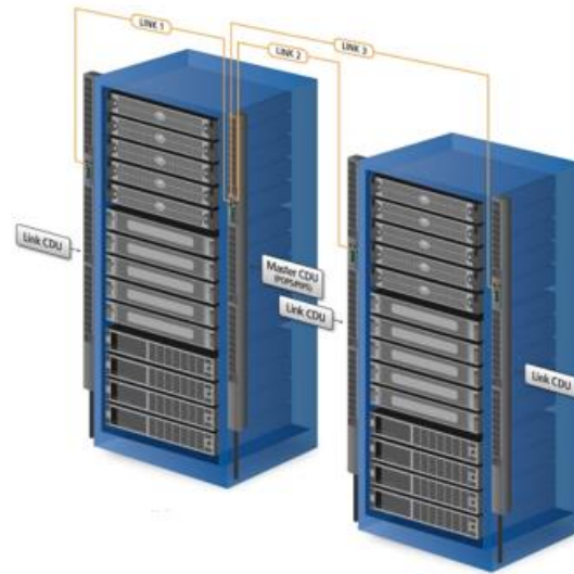
Multi-Linking View in the Equipment Cabinet
